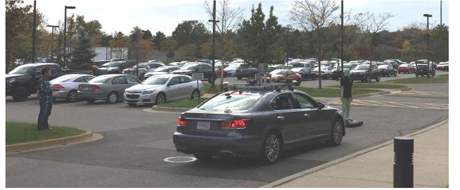
Fig. 5: Robotic pedestrian surrogate target with a Toyota autonomous vehicle.
